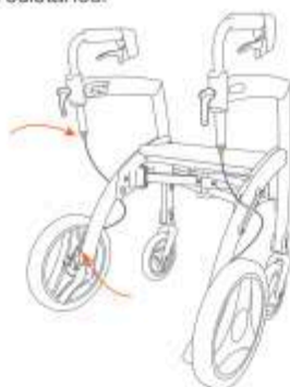
Figure 56: Brake adjustment via the adjustment screws at the top and bottom of the brake cable.
