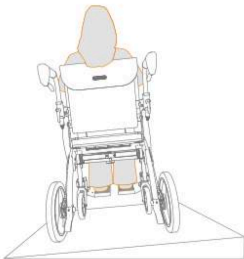
Figure 52: The maximum lateral slope angle is 3.5^\circ .
